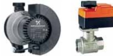
Variable speed pump or motorized modulating valve delivers variable water-flow, controlled by DXM2 control, based on loop water ΔT.
