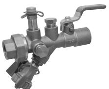
The valve is provided with a drain valve, which after installation should be vertically below the main valve and at its lowest point. This is a 90° operation ball valve providing positive isolation. The drain valve should always be set in the closed position – this is when the small lever is at 90° to the axis of the valve.
