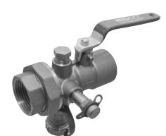
A drain valve is provided and after installation the drain valve should be vertically below the main valve. This is a 90° operation ball valve providing positive isolation. The drain valve should always be set in the closed position — this is when the small lever is at 90° to the axis of the valve.
