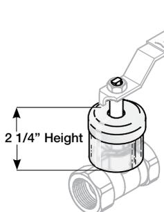
The "XH" stem extension is simple and effective design. This option is designed for installations where pipe insulation would make standard handles inoperable. The external plastic shield helps to keep the insulation away from the stem extension, providing years of trouble free operation.
