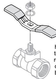
Tee handles offer the same installation space savings as oval handles, with a slightly shorter end to end dimension. Tee handles require more handle force to operate, so accidental openings can be reduced.
