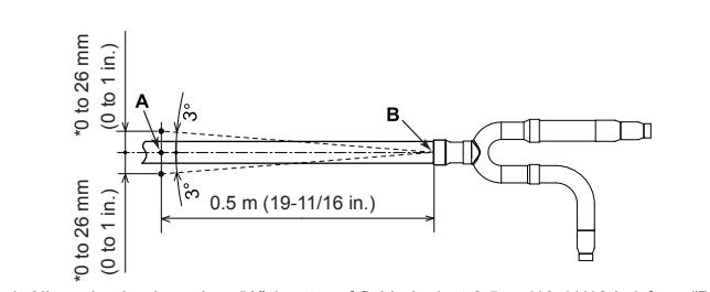
If the field pipe is connected with angle larger than specified, the balance of split refrigerant flow will be lost, and the refrigerant may concentrate upon specific outdoor unit as shown in the following figure. Such unbalanced refrigerant flow may cause a compressor malfunction.
