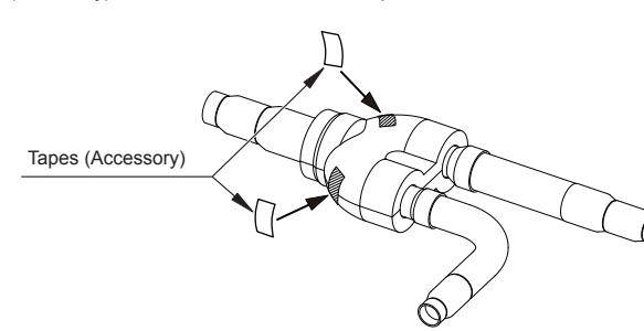
3) Use tape (Field supply) to seal the seam so that there will be gap at the junction between the aforementioned heat insulation and the heat insulation on the local piping.
