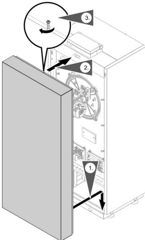
1. Place the front cover onto the locating pegs.
