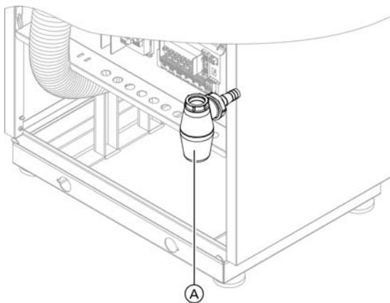
The Vitocrossal 300 CU3A boiler comes with a built-in condensate trap. An external trap is not required when connecting the field drain to the P-trap. Discharge tubing (field supplied) must be  $\frac{3}{4}$  in. diameter. Use CPVC, PVC or other material approved by code listed below.
