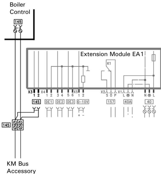
**Accessory kit for zone circuits or heating circuit with mixing valve connections**
