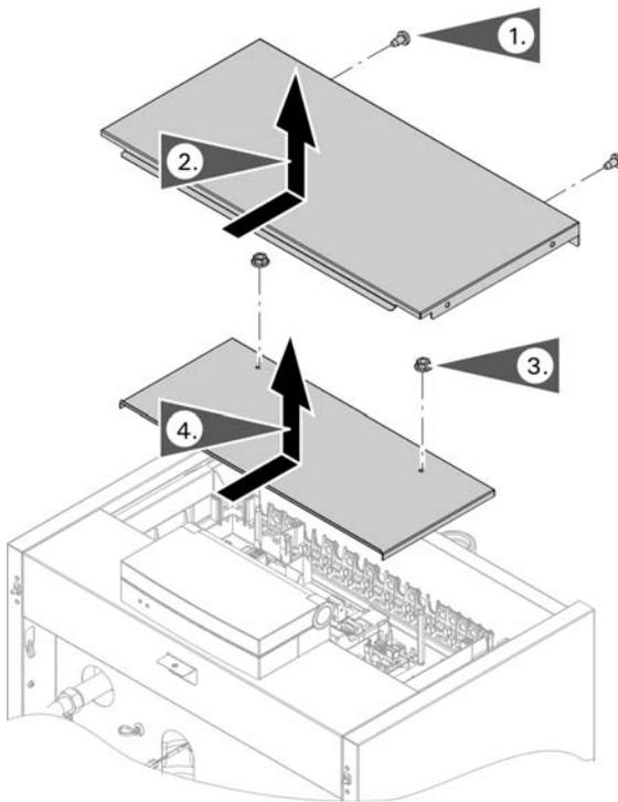
1. Remove the screws from the top panel and set aside.
