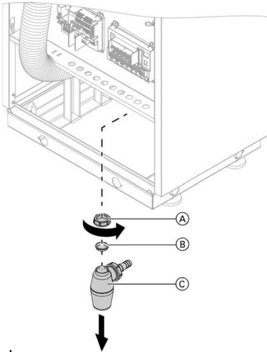
1. Remove the condensate siphon from the boiler.
