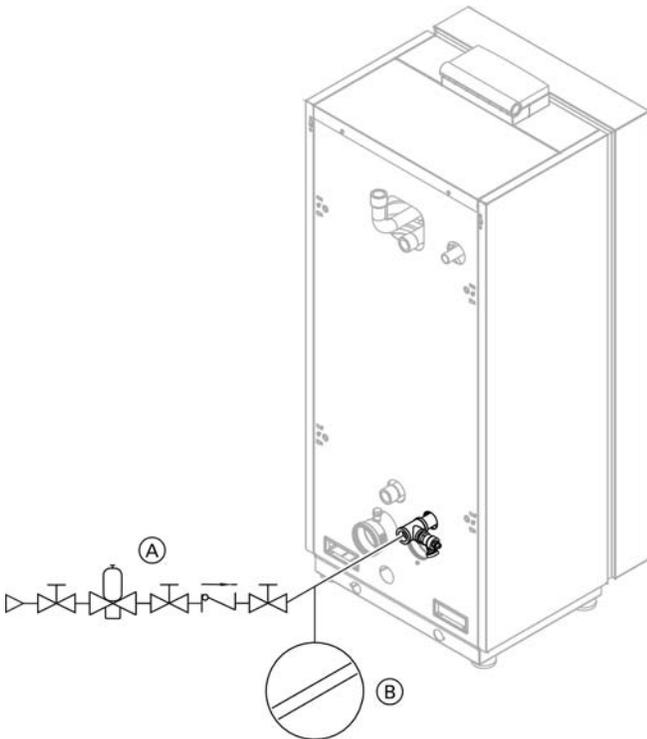
Installing boiler fill / expansion tank
