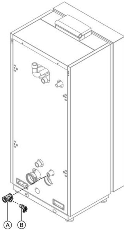
Installing drain valve
