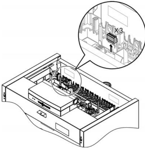
1. Remove the X3 plug from the control board. Attach sensors and reinsert the X3 plug. Refer to the following sensor information.
