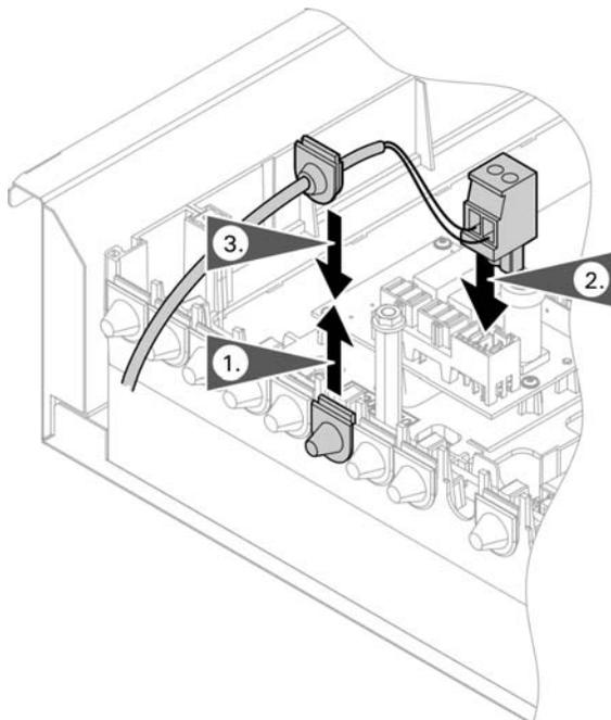
**Cables with moulded strain relief**
