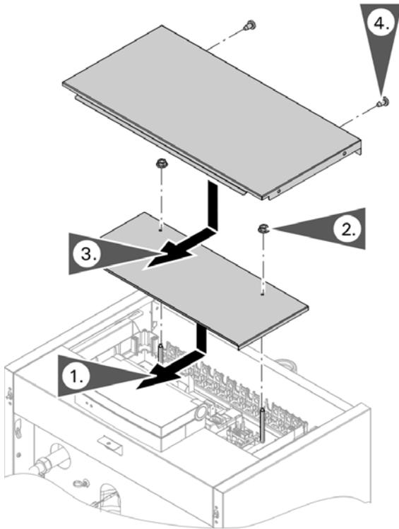
1. Place the control cover on the control connection housing and slide into place.
