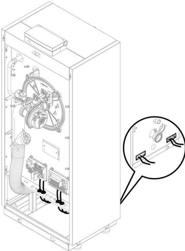
**Routing power/pump accessory cables**
