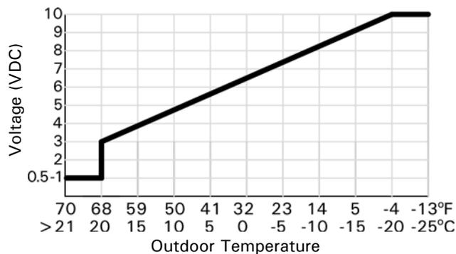
The chart is based on coding address E6 adjusted to 100.
