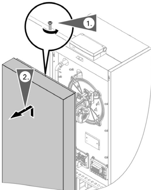
1. Remove the retaining screw and set aside.
