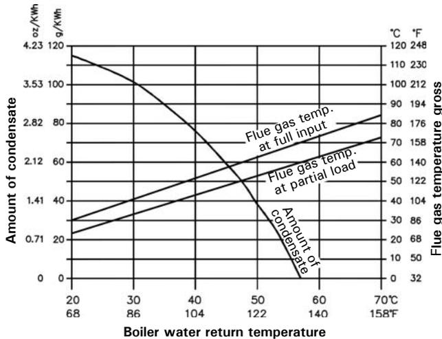
**Note:** The ‘amount of condensate’ and the ‘flue gas temperature gross’ graphs are independent of each other.
