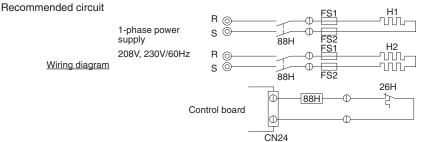
FS1, 2 ---- Thermal fuse H1. H2 ---- Heater 26H ----- Overheat protection thermostat 88H ----- Electromagnetic contactor
