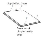
On original RETURN DUCT COVER, apply ¼" (6mm.) continuous bead of 500°F RTV sealant around flange (opposite insulation side), as shown.
