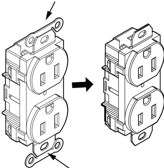
**NOTE:** If you don't see the perforation it might be necessary to snip the pieces off with a cutting tool. Avoid removing too much strap to maintain the integrity of the device mounting holes.
