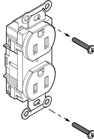
**STEP 3.** Prepare the device for mounting by removing the ears from the mounting strap or yoke by bending back and forth a few times at the perforation. For most receptacle also remove the ends of the strap at the perforation.
