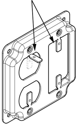
**STEP 2.** Remove and retain the mounting screws included with the device. These screws will be used to secure the device to the cover.
