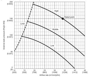
PEAD-A36AA7 (External static pressure 70Pa) 208-230V 60Hz
