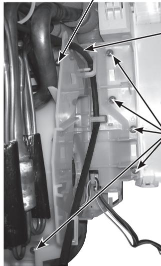
Lead wire of pipe thermistor
