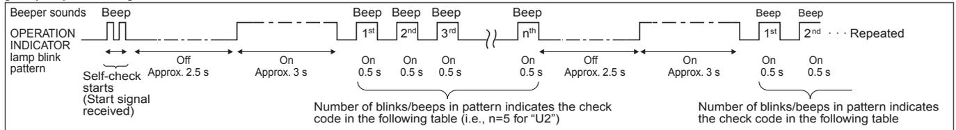
[Output pattern A] Errors detected by indoor unit
