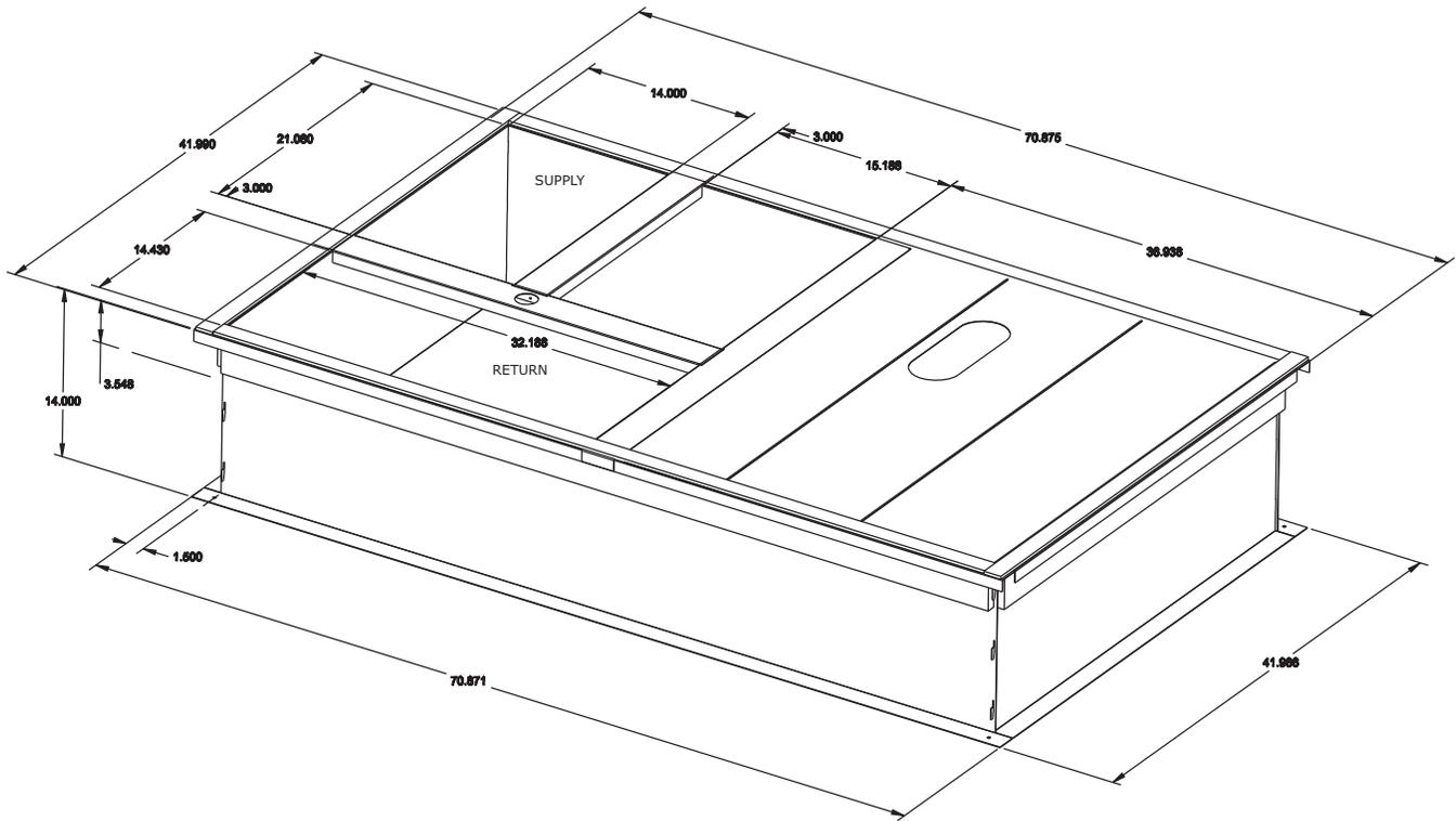
Figure 6. Cooling with optional electric heat and gas/electric models – downflow unit clearance – 15-25 tons
