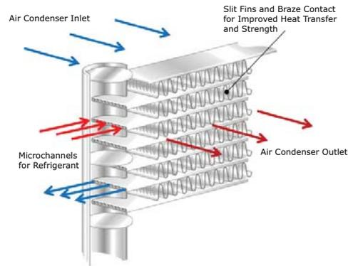
Microchannel coils are all-aluminum coils with fully-brazed construction. This design reduces risk of leaks and provides increased coil rigidity — making them more rugged on the jobsite. Their flat streamlined tubes with small ports and metallurgical tube-to-fin bond allow for exceptional heat transfer.
