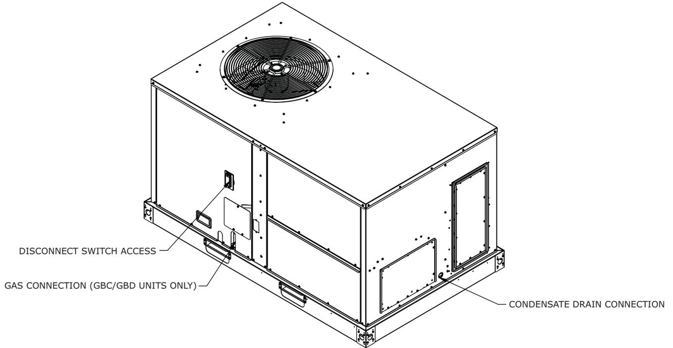
**Figure 2. Cooling with optional electrical heat and gas/electric units — front & side views — 3-5 tons**
