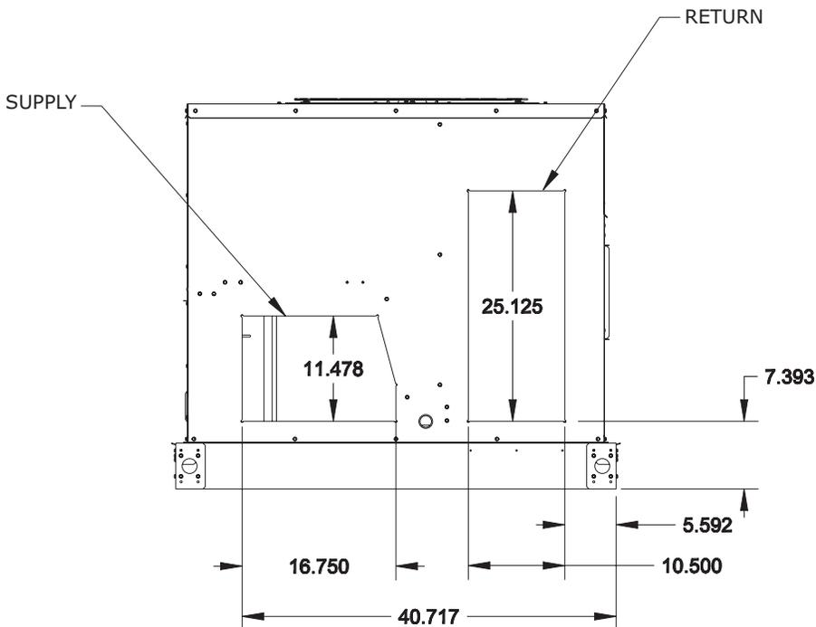
Figure 5. Cooling with optional electric heat and gas/electric models – roof curb – 3-5 tons
