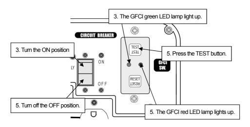
Press the GFCI RESET button.The GFCI green LED lamp lights up.
