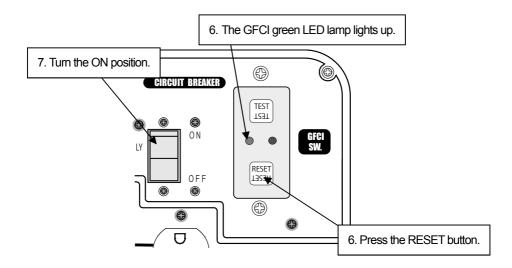
During generator use, if the GFCI RESET button extends and the circuit breaker trips, this usually indicates a faulty power tool, appliance, or cord.
