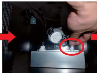
Unplug light unit assembly connector, Then take out the whole assembly
