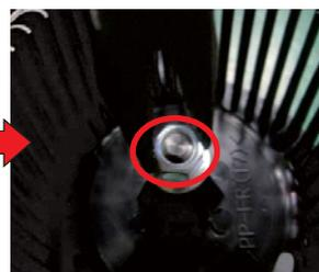
Remove the blade fixing nut
