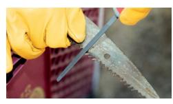
For sharpening crosscut saws, circular saws and saw teeth with less than 60° angle.
