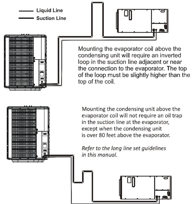
Insulation is necessary to prevent condensation from forming and dropping from the suction line. Armflex (or satisfactory equivalent) with 3/8" min. wall thickness is recommended. In severe conditions (hot, high humidity areas) 1/2" insulation may be required. Insulation must be installed in a manner which protects tubing from damage and contamination.
