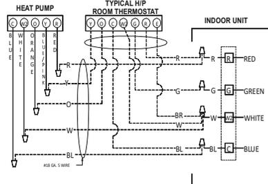
SYSTEM COMPOSITE DIAGRAM - HEAT PUMPS - ABOVE 10 KW
