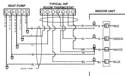
SYSTEM COMPOSITE DIAGRAM - ALL SIZES (EXCEPT 5T 16SEER) HEAT PUMPS - ABOVE 10 KW
