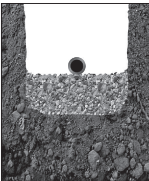
Trench in bad soil
