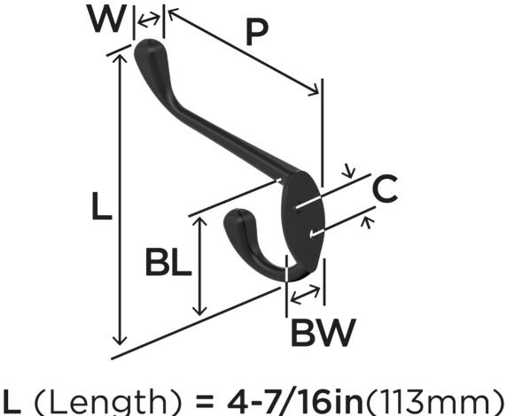
**C** (Center-to-Center) = **11/16in**(17mm) **BL** (Base Length) = **1-7/8in**(48mm)
