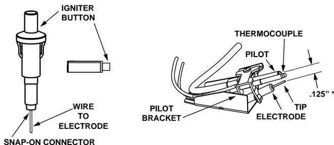
\* NOTE: SPARK GAP DISTANCE MEASURED FROM ELECTRODE TIP TO PILOT.
