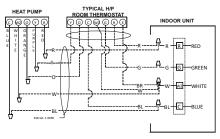
SYSTEM COMPOSITE DIAGRAM - ALL SIZES (EXCEPT 5T 16SEER) HEAT PUMPS - ABOVE 10 KW
