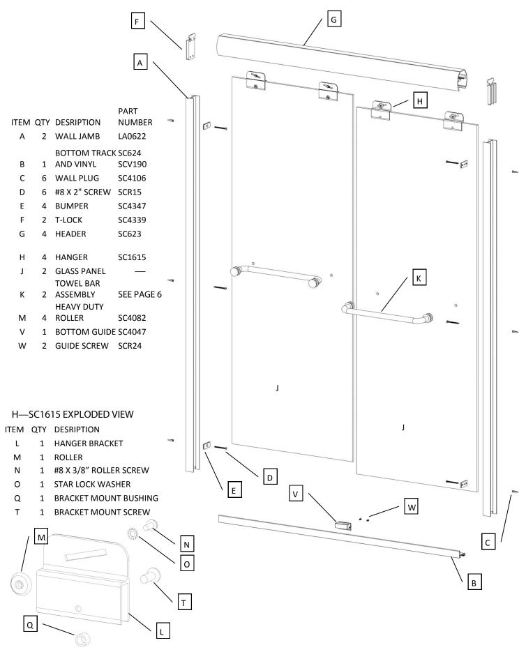
1 This framess bypass sliding enclosure is supplied with custom fit **Wall Jambs [A]**. The jambs are notched one end to fit over the bottom track.
