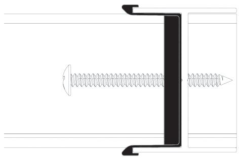
**NOTE:** Be sure that the ears on the bumper install over the wings of the wall jamb
