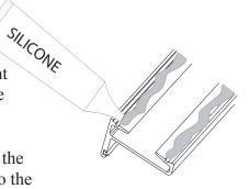
Alternative Method: Run 2 beads of silicone inside the pnecil marks on the threshold. Place the tub track in position over the silicone, lining it up with the pencil marks on the threshold from the previous step.
