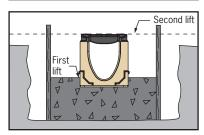
Concrete should be poured evenly (both sides of channel) and carefully to avoid dislodging channels. A wand type concrete vibrator should be used to ensure concrete distributes evenly around channels.
