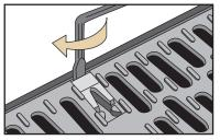
Rotate through 90° until lock mechanism slides across and clicks open.
