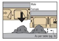
d) Lower channel vertically onto 'patties' and position to correct height and alignment ensuring 'tight' connection to previous channel.
