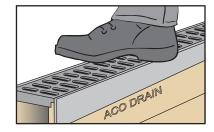
To remove first grate, insert removal tool under grate bar, pull up sharply. Subsequent grates can be removed by hand - Grip end of grate and lift sharply.
