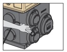
Attach outlet pipe using coupler, if required seal using appropriate sealant/adhesive. If corrosive liquids are transported in trench, ensure sealant or adhesive is chemically resistant.
