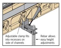
Create required width template using timber sheet or similarly suitable rigid material. Diagrams can be printed from the ACO website.
