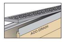
To install grate, align clips in underside of grate with recesses in edge rail. Push down/stand on grate until clicks into position.
