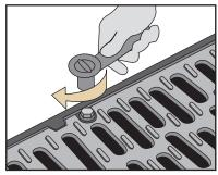
2. **To unlock:** use wrench or socket set to loosen/remove bolts. Use grate removal tool to lift first grate, sliding from beneath anti-shunt lugs. Once unbolted, other grates can be removed by hand (use gloves).
