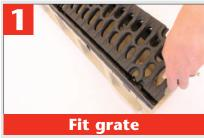
Position grate onto channel, align holes in grate with matching holes in edge rail. Using wrench or socket set to tighten. If using a torque wrench, do not set to more than 15 ft. lbs.
