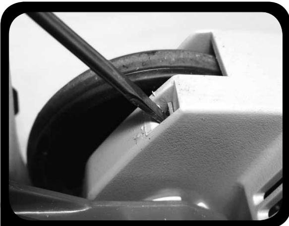
3. If there is not enough detent spring to remove with pliers use a flat head screwdriver to pry out broken spring.
