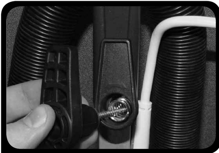
3. Insert impact bumper assembly into cord wrap bracket.
