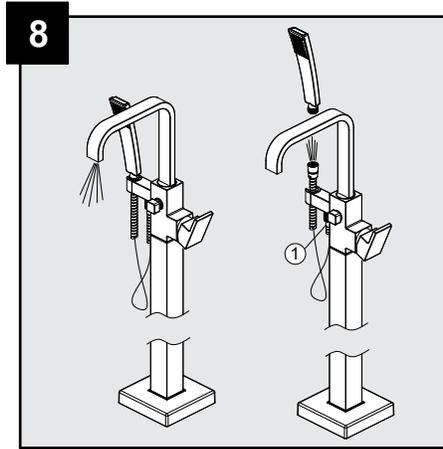
Flushing debris and checking for water leaks:
