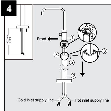
Attach the mixer (1) to the standpipe (2), make sure the prongs (3) on the standpipe (2) insert into the hole (4) of the mixer (1). Install the set screw (5) and tighten into the standpipe (2) with hex wrench.
