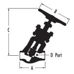
Class 2500 • Full Port—Y Pattern—Welded Bonnet—Threaded and Socketweld Ends
