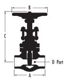
Class 800 • Standard Port – Welded Bonnet – OS&Y Threaded and Socketweld Ends
