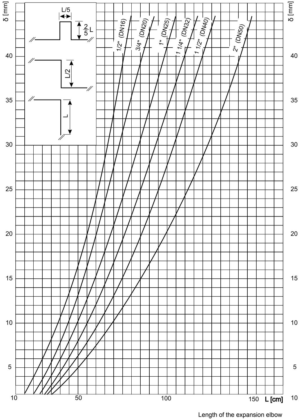
**EXAMPLES OF DETERMINATION OF THE COMPENSATING ARM L for PVC-C at  $t_i = 55^\circ\text{C}$ ,  $t_m = 10^\circ\text{C}$**
