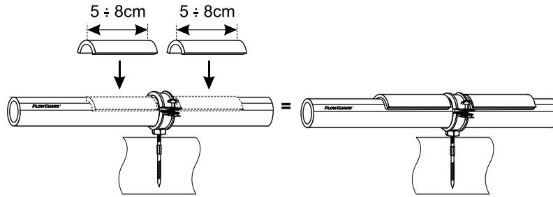
**Fig. 15. Fixed support on pipe (using cement)**
