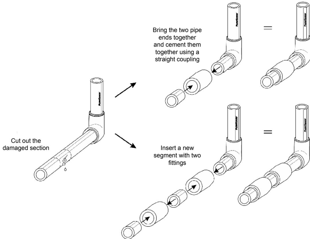
When leakage occurs at the fitting, the best repair method is to cut off the fitting with sections of the pipe and insert a new pipe with two fittings.
