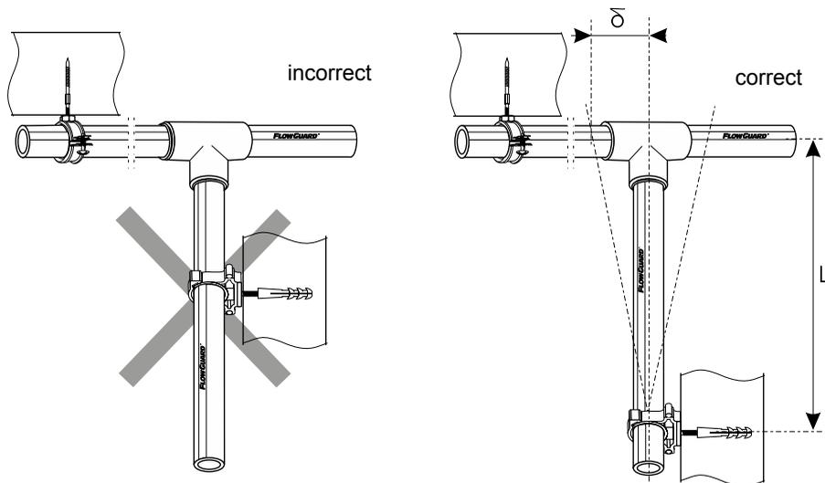
Fig. 14. Correct and incorrect inclusion of an expansion elbow
