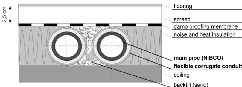
**Fig. 13. Laying installation in a flexible corrugate conduit (e.g. through ceiling)**
