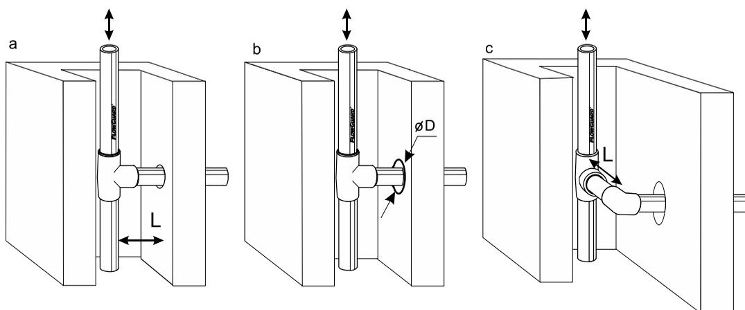
**Fig. 9. Compensation of thermal expansion in vertical ducts**
