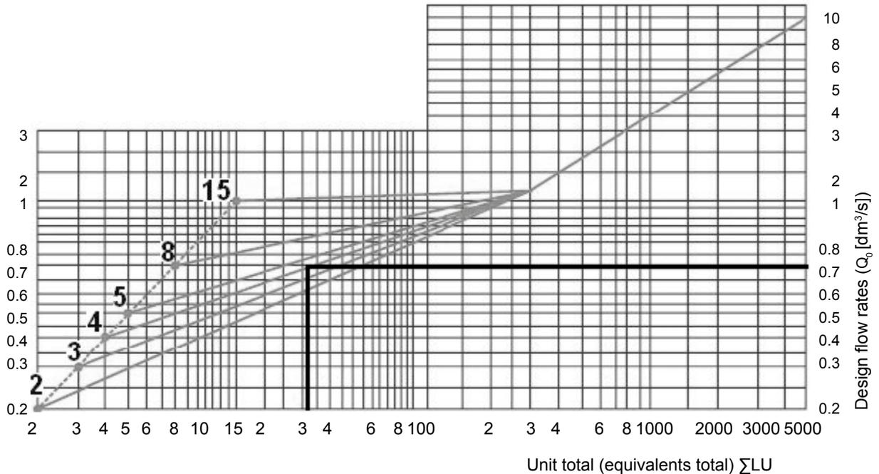
**Fig. 1. Nomograph for determining design water flow rates in water distribution systems ( $Q_o$  [dm<sup>3</sup>/s]), depending on the total of equivalent load units ( $\Sigma LU$ )**
