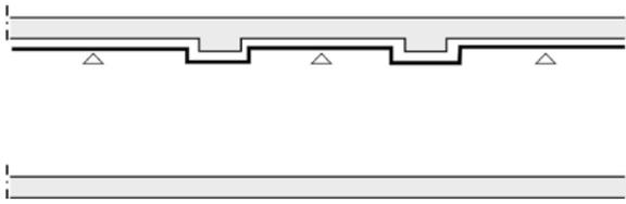
Fig. 19. Locations of the pipe and supports under a ceiling – sectional view
