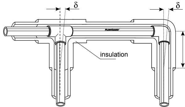
**Fig. 11. Bend area insulation**
