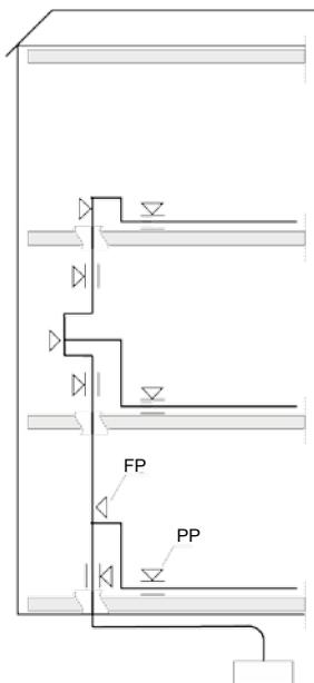
**Fig. 17. Locations of fixing supports in service drop**
