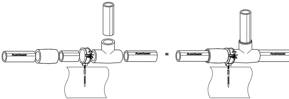
**Fig. 16. Fixed support on pipe (using fittings)**
