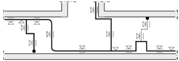
Fig. 20. Locations of the pipe and supports – layout
