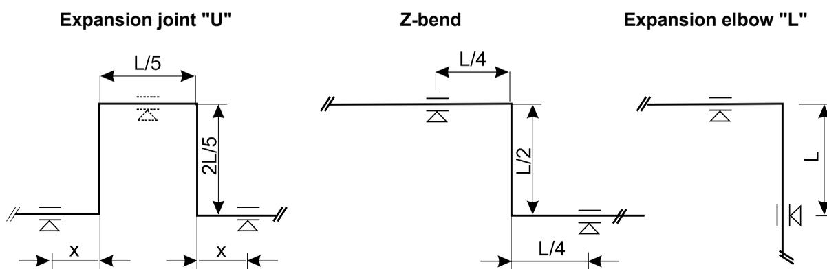
**Fig. 6. Expansion joint types**
