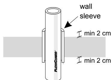
**Fig. 10. Penetration through construction partitions**
