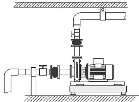
Fig. 21. Installing the pump
