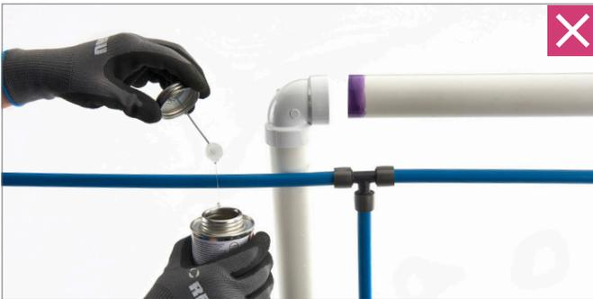
Ensure that the employed sealants, cleaning agents, building foams, insulation, protective tape, adhesive tape or thread sealant do not contain any components which cause stress cracking or corrosion, such as ammonia, ammonia-bearing, aromatic and oxygenated solvents (e.g., ketone and ether), chlorinated hydrocarbons or chloride ions which can leach.
