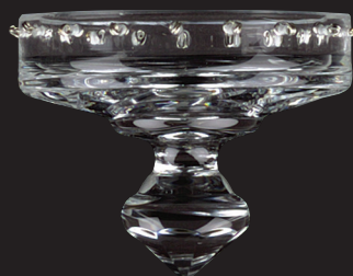
Bottom Piece Clear • Hand Cut and Polished with 18 pins Attaches by Pin Hole Connectors Diameter 75mm • Height 63mm Inside Diameter 69mm • Chrome Pins
