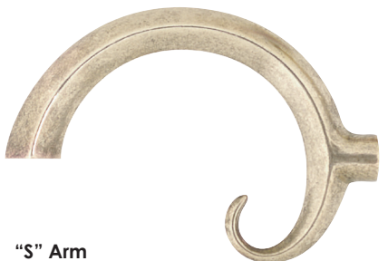
"S" Arm Spread 4-7/8" • Height 3-1/8" Tapped 1/8 IPS both ends with wireway E5303 ..... Unfinished
