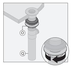
**Note:** Make sure flange is centered in drain opening.
