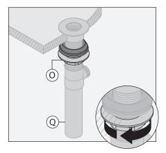
**Note:** Make sure flange is centered in drain opening.
