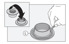
5) Insert flange (L) into drain opening. From below, attach drain body (Q) with gasket (M) and washer (N) to flange (2-3 turns until hand tight).
