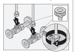
**Optional:** Adjust limit stop washer to limit handle turn to the hot position if desirable.
