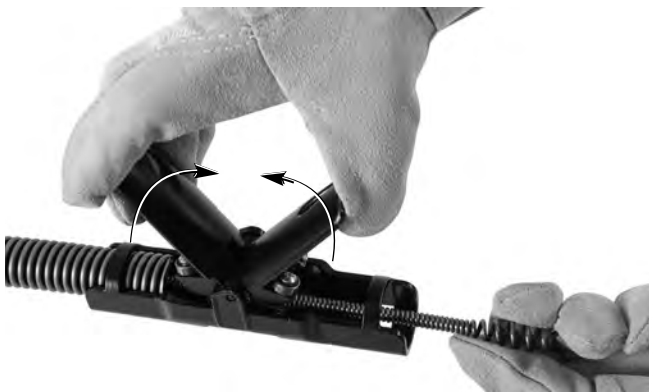
Figure 5 – Feeding Cable Through AUTOFEED® Assembly
