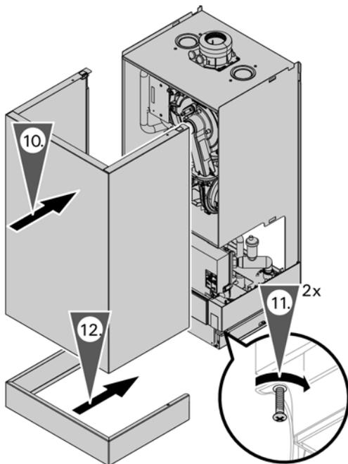
10. Set front enclosure panel on the guide rails and push in place.
