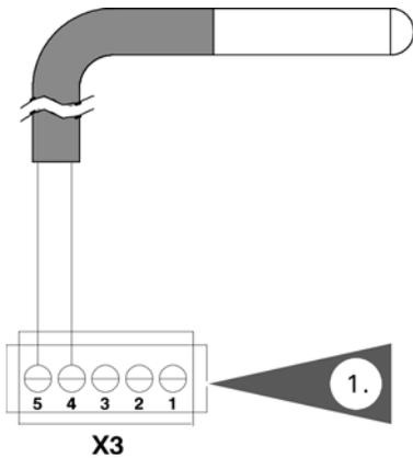
1. Connect the low-loss header sensor (if LLH is used) to terminals X3.4/X3.5 on the boiler control board.
