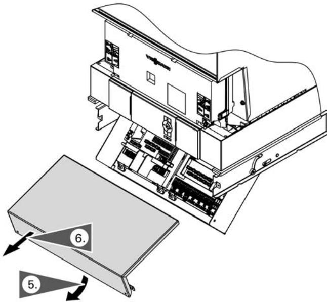
5. Tilt the bottom of the external accessory connection box cover forward.
