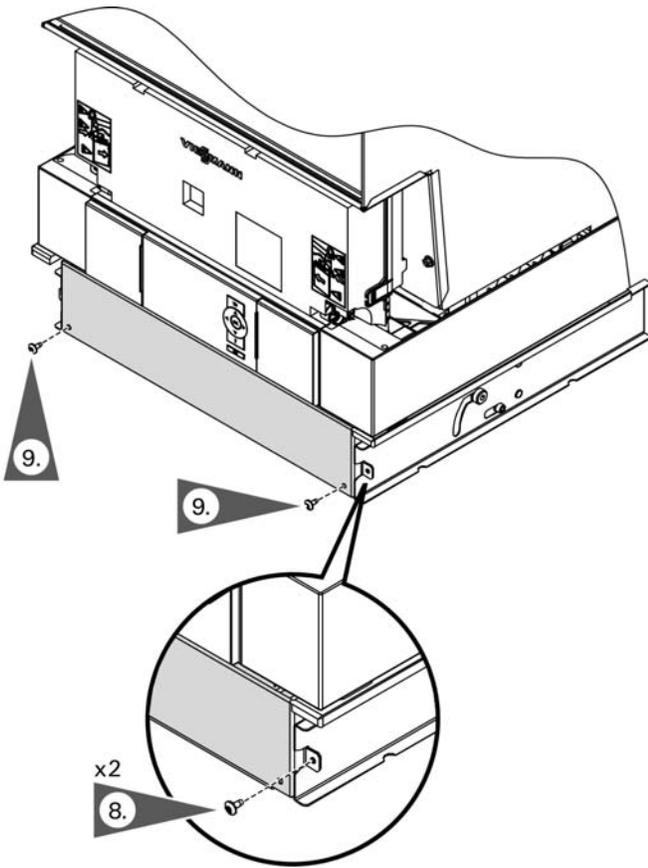
8. Tighten the external accessory connection box retaining screw.
