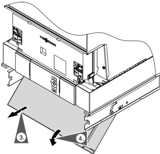
3. Pull the external accessory connection box forward until the retaining screws are clear of the guides (built into the rails).
