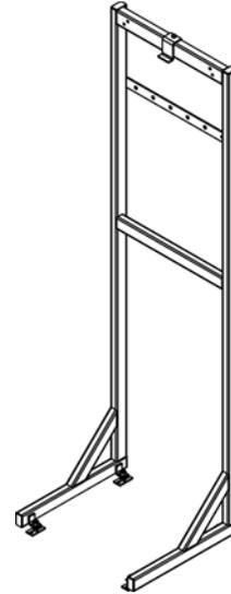
The Vitodens 200-W, model B2HB does not come with a mounting template. The wall location for the frame, mounting bracket and all vents must be field calculated.
