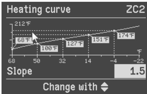
Example: Changing the heating curve slope to 1.5
