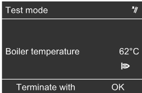
Emissions test mode should only be activated by a certified technician during the annual inspection.
