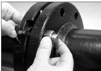
6a. Thread standard flange nuts finger-tight onto the two mating bolts.
