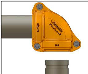
**5. INSERT SECOND MATING COMPONENT END:** Insert the second grooved mating component end into the other opening of the fitting. The grooved mating component end shall be inserted into the fitting until contact with the pipe stop of the gasket occurs. A visual check is required to verify that the fitting's keys align with the groove in the mating component end.
