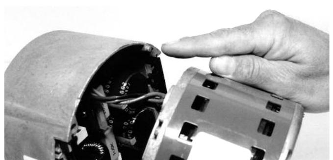
4. Locate the two standard 1/4" hex head bolts on the flat end of the motor control module casting. Remove these bolts from the motor while holding the control module. **DO NOT REMOVE TWO SCREWS WITH TORX HEADS.**
