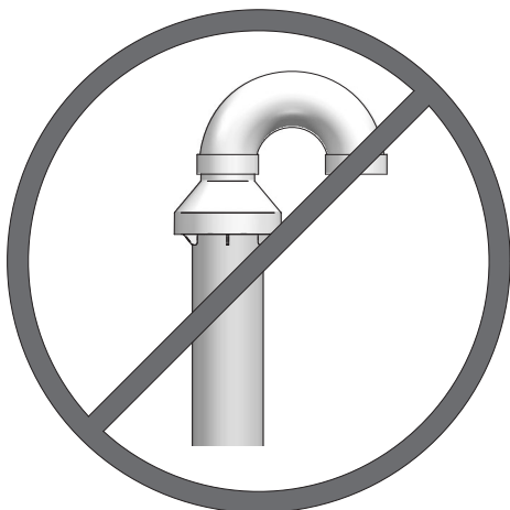
Figure 5-5 Do Not Install U-Bend to Rain Cap
