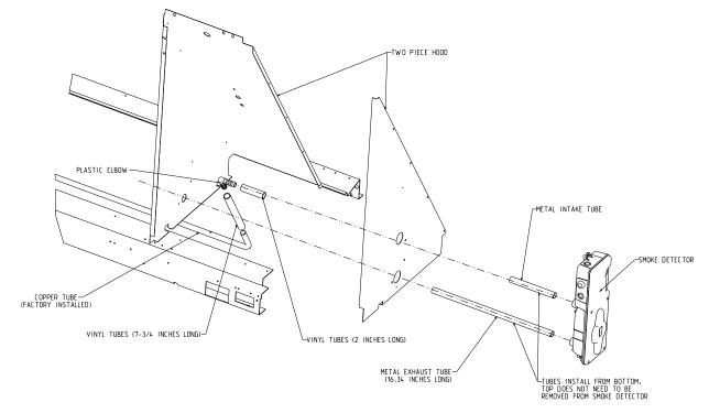
Figure 25. Return air smoke detector for downflow units
