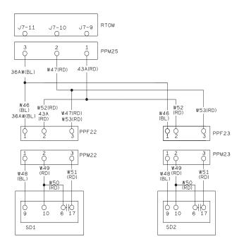
WIRING INSTRUCTIONS: 1. CONNECT PLUGS TOGETHER AS SHOWN.
