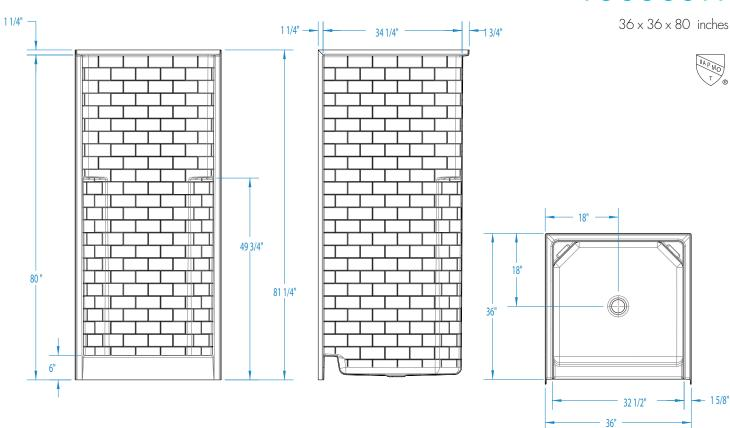
FEATURES Ibs Dimensional Tolerance ± %". Dimensions needed for site preparation should be measured from the unit. Aquatic assumes no responsibility for preparatory work.
