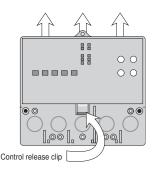
Press the control release clip on the base inside the wiring chamber and slide the control upwards.
