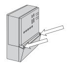
Loosen the screws at the front of the wiring cover.
