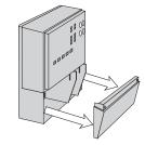
The wiring cover pulls straight out from the wiring chamber.
