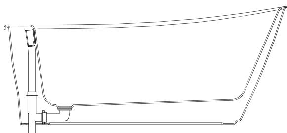
Standard drainpipe and overflow compatible with end-drain freestanding bathtub models: 105571 (Optik 60") and 106266 (Ariosa 60").
