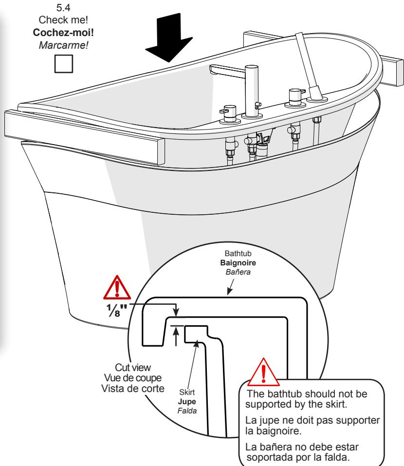
To complete the installation and solidify the bathtub, apply a bead of silicone along the seam where the bathtub rests against the skirt.
