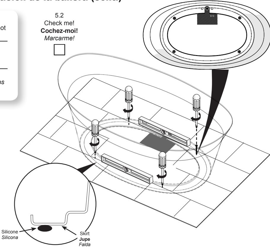
Add two spacers (example 2x4) on the skirt ends and position the bathtub inside the skirt. Attach the hot and cold water riser to the plumbing hoses.
