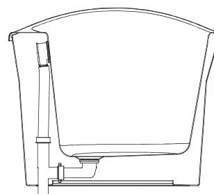
Standard drainpipe and overflow compatible with center drain freestanding bathtub model: 105742 (Optik 66") and 106267 (Ariosa 66").
