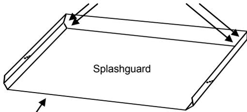
Open end of splashguard should rest on the horizontal drain pan.
