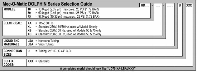
Junction Box option is available on 230V models at no additional charge. Contact the factory for model numbers. Shipping weight for Dolphin Pumps is 7 lbs.
