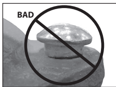
OVAL NECK OF BOLT NOT SEATED PROPERLY
