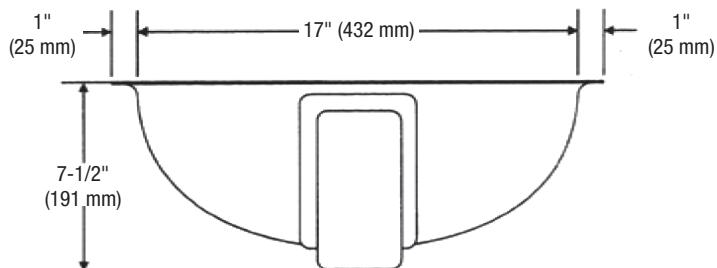
Note: All dimensions and specifications are nominal and may vary: Dimensions of 8" and greater have a tolerance of +3%. Dimensions less than 8" have a tolerance of +5%. Please utilize the current cutout template for countertop cutouts.
