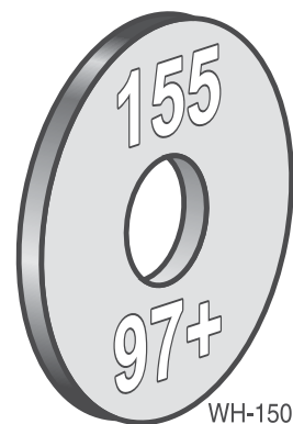
Figure 16 Propane gas orifice identification ECO 155
