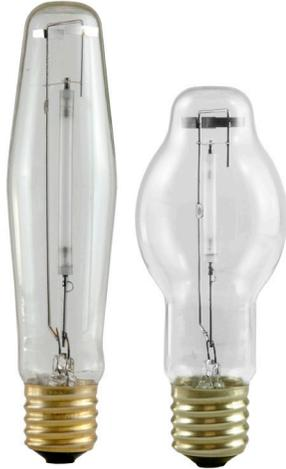
The SYLVANIA LUMALUX PLUS and LUMALUX PLUS ECO lamps incorporate the latest technology to eliminate the end-of-life cycling of HPS lamps. They remain off at end-of-life. LUMALUX PLUS/ECO lamps are constructed with lead-free welded bases and pass the existing Federal TCLP test.
