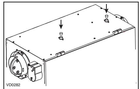
Insert both drain plugs (included in parts bag) in alternate drain fittings located on top of the unit.
