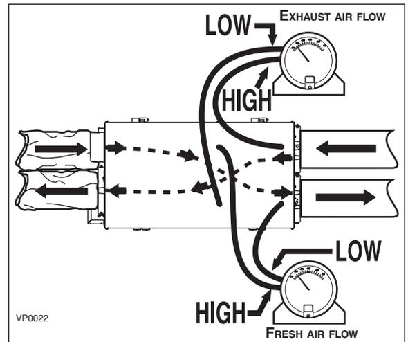
NOTES: 1. Use conversion chart provided with the unit to convert magnehelic gauge readings to equivalent cfm values.
