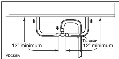
Cut 2 sections of plastic tube, at least 12"-long each, and attach them to each inner drain fitting, located under the unit.
