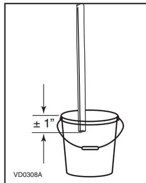
Run the tube to the floor drain or to an alternative drain pipe or pail.
