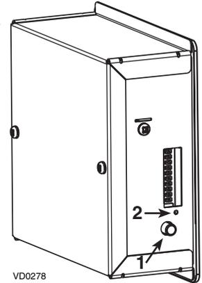
If a problem occurs during the unit operation, its integrated control LED (2) will blink. The color of the blinking light depends on the type of error detected. Refer to Section 9 Troubleshooting on pages 19 and 20 for further details.
