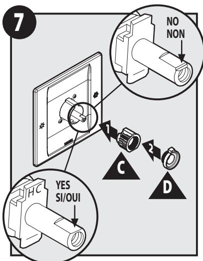
Make sure cartridge stem is positioned with notch facing down. Insert Key Stop (C) & Adjustable Limit Stop (D) into Stop Tube.
