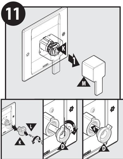
Remove the Lever (M) and Lever Handle Adapter (K). Note the position on the stop. Position the Adjustable Temperature Limit Stop (D) so the Lever stops at the position. This prevents the Lever from being turned into an unsafe temperature.
