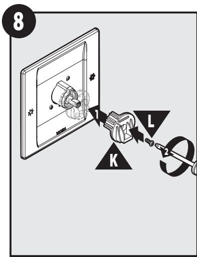
Install Handle Adapter (K) onto cartridge stem with Handle Adapter Screw (L).
