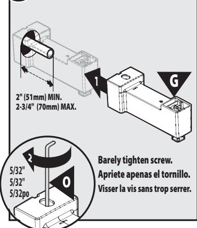
1. Install Tub Spout (G) upside down onto pipe.
