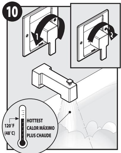
1. Turn handle on to test hot water temperature.
