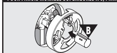
Slide Stop Tube (B) onto valve.
