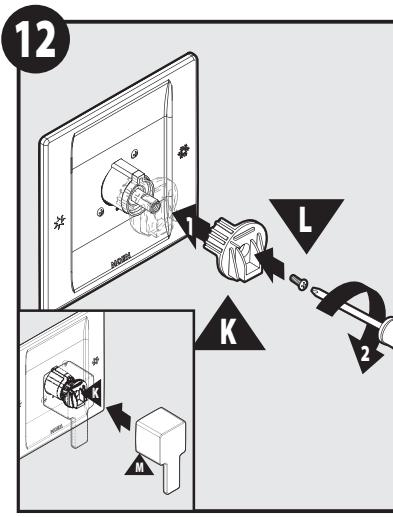
After setting the adjustable temperature limit stop to the desired position, reattach the Lever Handle Adapter (K), Adapter Screw (L), and Lever (M). Make sure ridges on back of (K) are to the left of the tab on (D).
