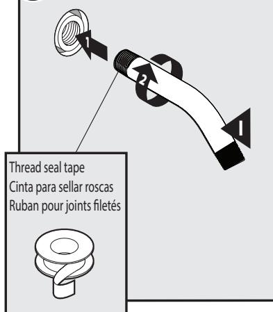
Wrap thread seal tape around Shower Arm (I) threads. Screw Shower Arm into connection in wall.
