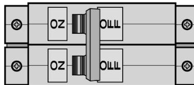
**For use on an individual branch circuit only.** The heater shall be installed using insulated, UL listed, 2 wire cable (2 wire plus ground) of the appropriate size suitable for up to 75°C and protected by the correctly rated circuit breaker.
