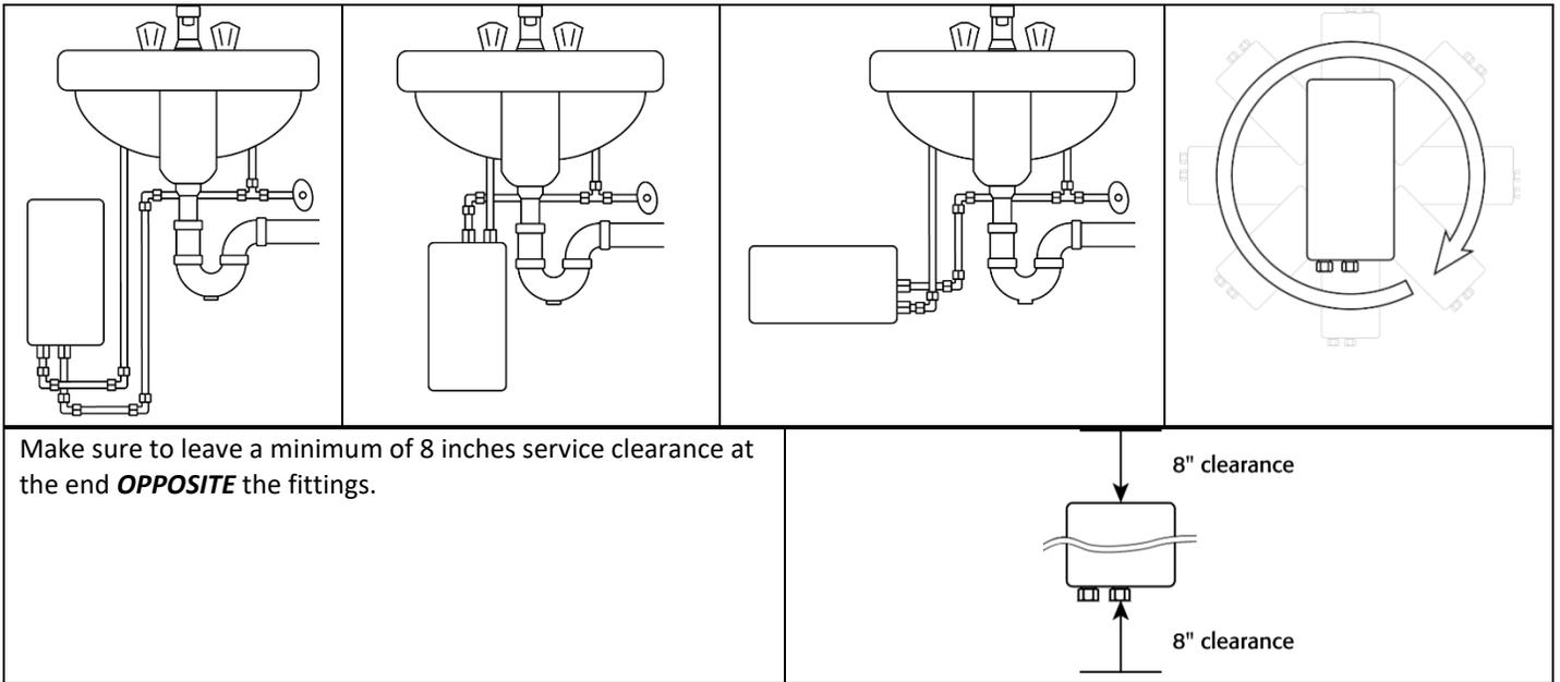
Remove the cover and fasten to the wall using the mounting holes at each corner of the back plate. Replace the cover.
