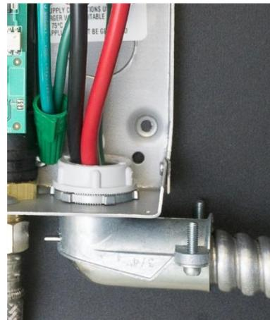
The power leads are to be secured to the L1 and L2 or L and N connectors on the terminal block or relay. The ground lead is to be secured to the GND connector on the block or the green ground wire with the provided wire nut.
