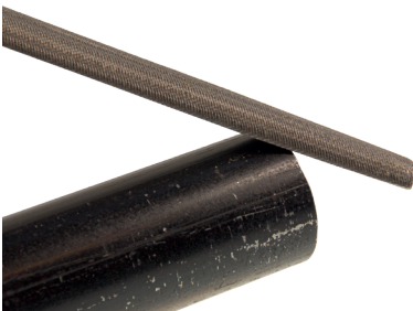
FIGURE 7: DEBURRING THE PIPE
